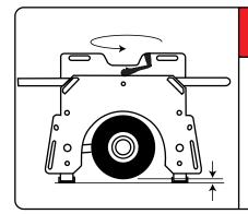
WARNING PROPER SETUP REQUIRES THAT WHEELS MUST BE OFF THE SURFACE AND SPIN FREELY PRIOR TO USE
