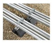
Strut model PipeGuard units are designed to support multiple pipes up to 6-inches (152 mm) in diameter at heights from 4- to 10-inches (102 to 254 mm) above the roof. Each strut model features a low profile, 1 5/8-inch (41 mm) wide galvanized strut channel designed to accommodate single or multiple strut clamps (sold separately).
